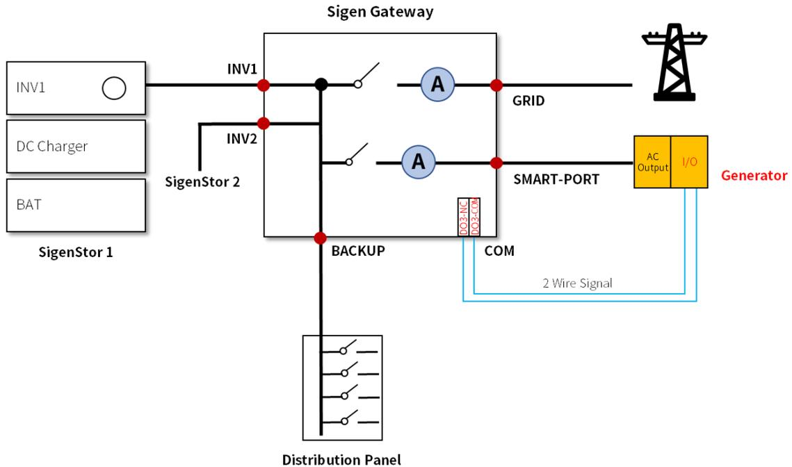
Generator two-wire start: Generator power output is connected to the SMART-PORT port of the Gateway. Generator DI port (please refer to the generator manual) is connected to the DO3-NC and DO3-COM ports of the Gateway control board. In this way, you can control the start and stop of the generator.
