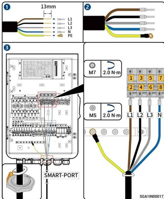
Follow the instructions in the diagram above to connect the Generator power wires to the Gateway's SMART-PORT circuit breaker. Then refer to the user manual of Gateway, switch off all circuit breakers and wait for at least 5 minutes before connecting the wires, and then switch on the circuit breakers one by one.
