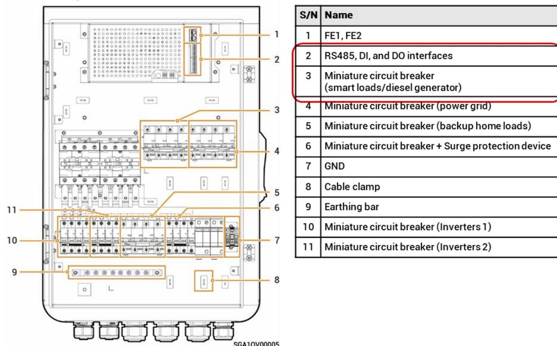
Confirm generator-related circuit breaker and I/O control port locations in the Gateway. As shown in the diagram above, NO. 3 is the generator power access circuit breaker and NO. 2 is the I/O control port of the Gateway.
