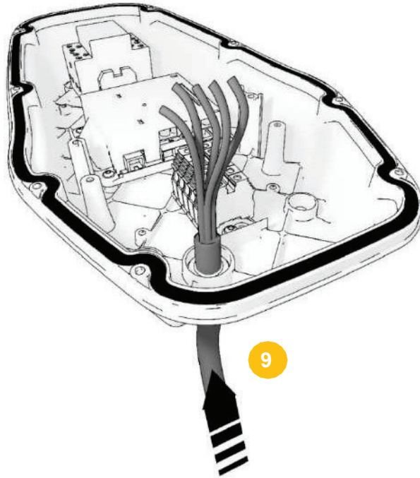
Figure 9 Cable entry supply line from behind
