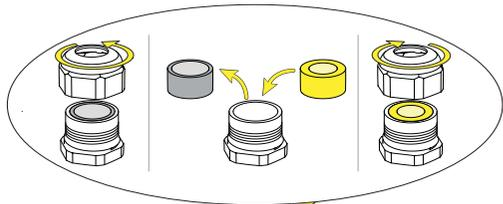
If the AC cable have a diameter between 20...26 mm should be installed the supplied reducing seal.
