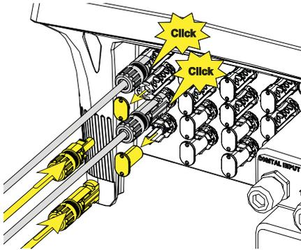
**ATTENTION** – Check that protective caps are installed on unused connectors. This is necessary for the inverter seal and to avoid any damage to the unused connectors which may be used at a later time.
