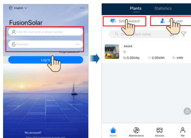
Figure 7-3 Creating a PV plant and a user
