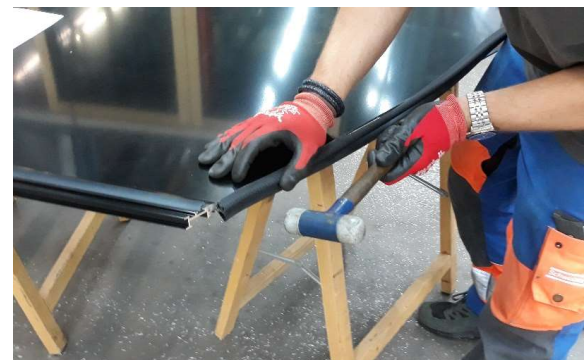
Fig. 13: Clip-on steel strip to finish the cut edge
