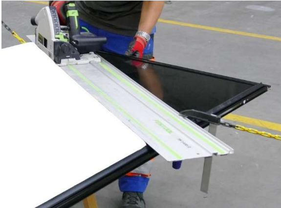
Fig. 8: Cutting the dummy module
