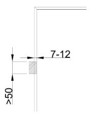
Installers must ensure that the resistance of the clamps is sufficient given the maximum pressure to which the module can be exposed. The clamps are not supplied by DualSun.
