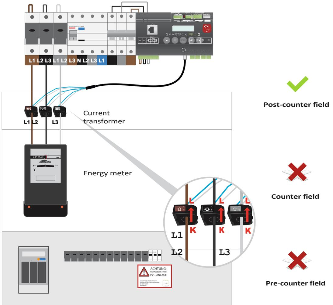
**Attention! The SMARTFOX current transformers must always be connected as shown in the picture above. (Arrows point in the direction of the consumer).**
