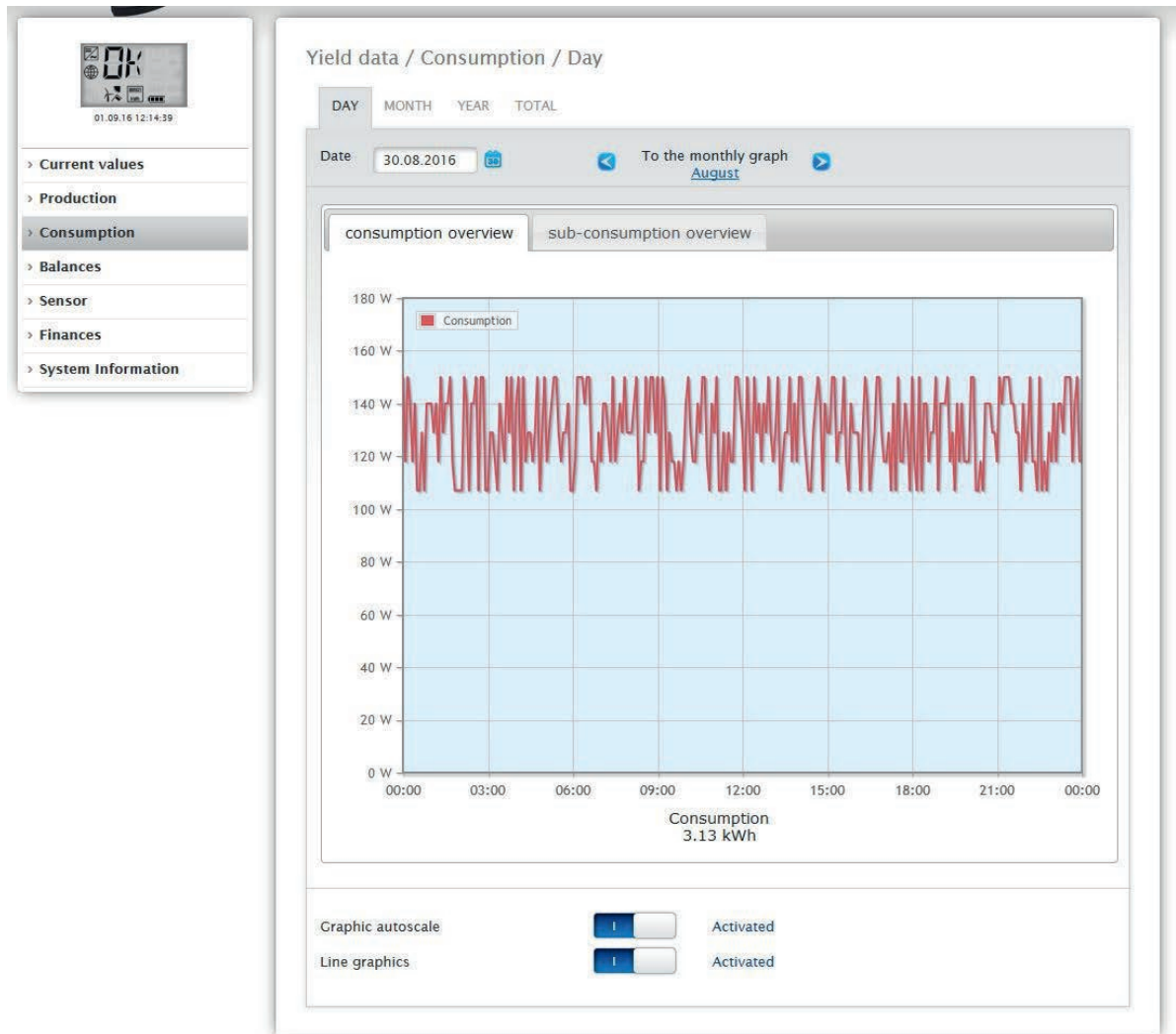
Fig.: Graph of daily consumption with meters connected and active line graphics
