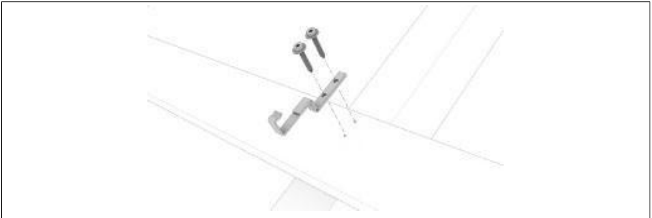
Image 4-5: Fastening mounting clamp “frame”
