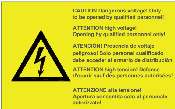
"Dangerous voltage" sticker
