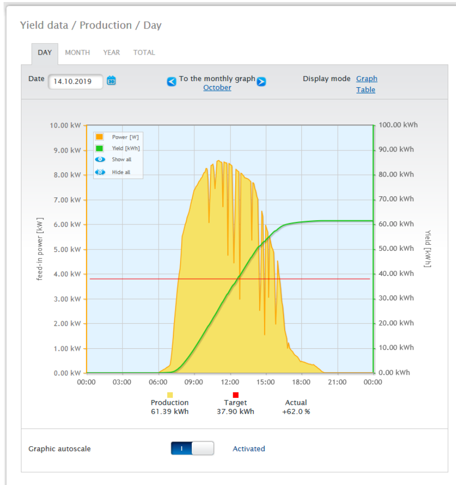
Fig.: Daily View of the Production Graph with the Auto Scaling activated
