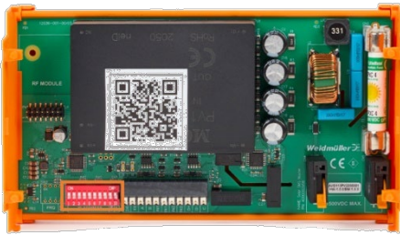
Figure 6.5 DIP switch (SW1) of Solar SMS master
