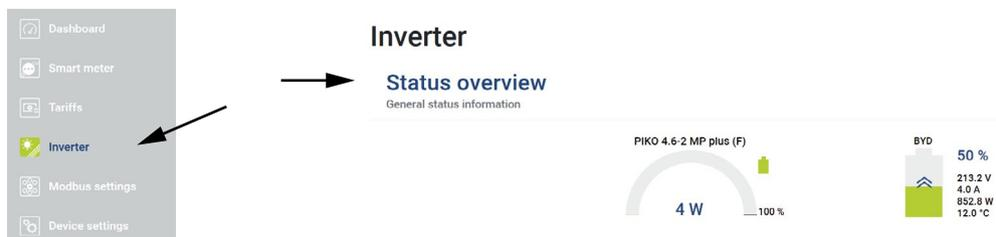
13. The two devices - inverter and battery - are displayed in the inverter view under „Devices“.
