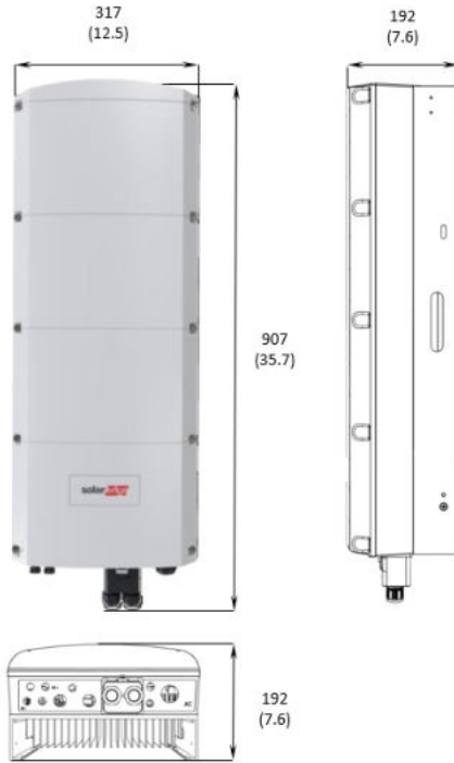
Figure 29: SolarEdge Home Hub Inverter - Three Phase: dimensions
