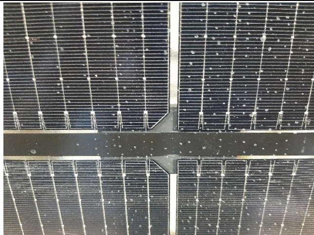
Example of break-through from cells to junction box
