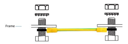
It is recommended to use a 10 mm² bonding connector to realize the grounding between each module. The recommended section to the main equipotential bonding is 16 mm².
