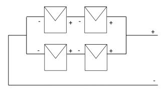
Note: When a project is wired with modules in parallel, it is important to check at the fuse rating of the module. This value is available on the module's label as well as on the dedicated data sheet. Indeed, in case of 1 line shadowing, the line that is still producing energy will "load" the other. This is why an appropriate line fuse protection must be applied and following appropriate standards.
