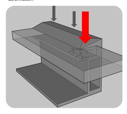
When clamping, please make sure that force is homogenous shared on aluminium part. Forced cannot deform top frame flange. For modules series equipped with a water drain corner, clamp must not be applied directly on.
